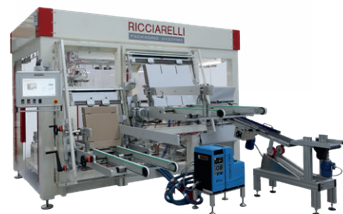
The new automatic casepacker mod. IWR22
